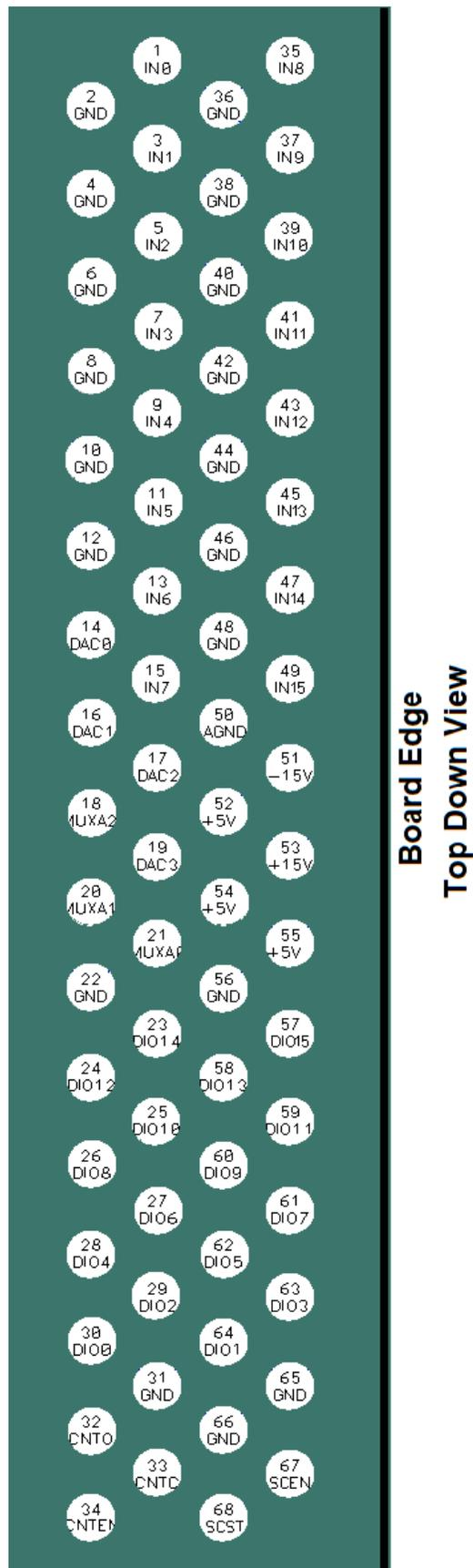
Figure 3-2: 68 Pin I/O Connector Footprint with Pin Numbers and Signal Names
