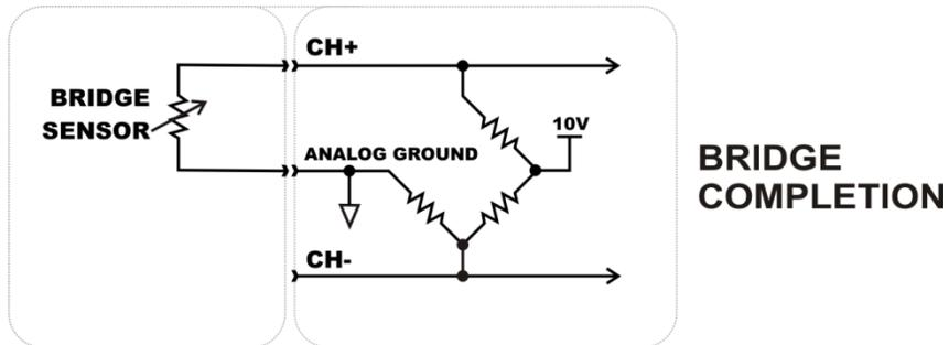
Figure 9-6: Bridge Completion Diagram
