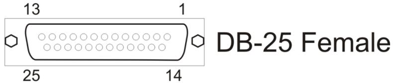
**Figure 9-11: J5 DB25 Female Connector Pin Locations**
