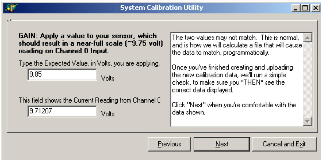
Figure A-5: System Calibration Utility Screenshot 4 (gain)
