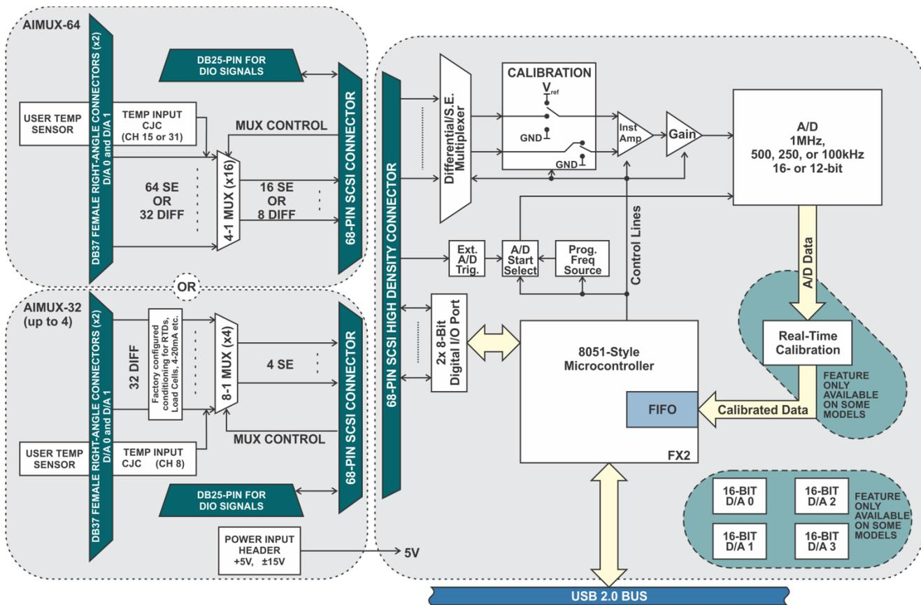
**Figure 9-1: Family Block Diagram showing AIMUX-32 and AIMUX-64**
