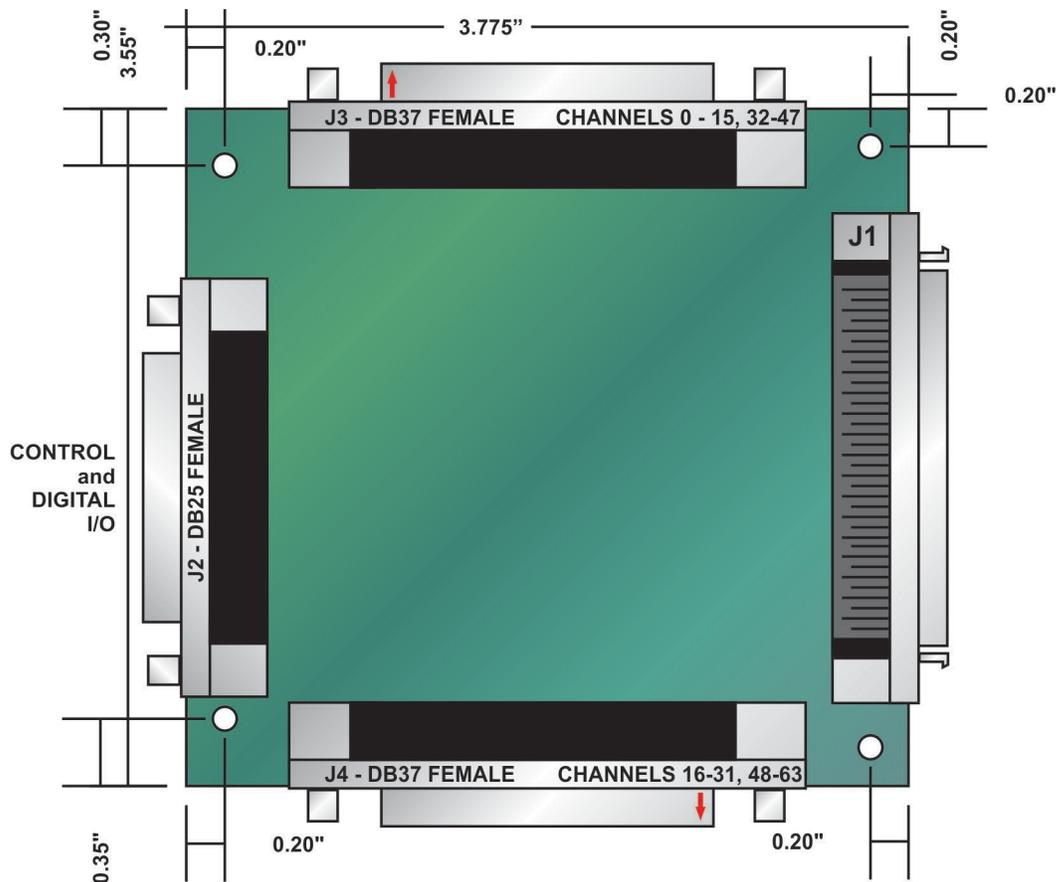
**Figure 8-1: AIMUX-64 Board with Connectors**
