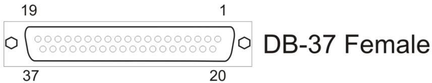
**Figure 8-2: 37-Pin Female Connector Pin Locations**
