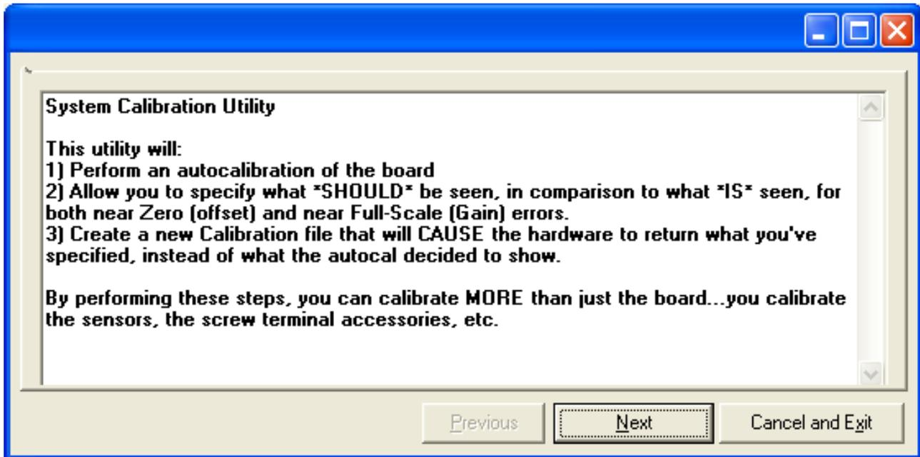
Figure A-2: System Calibration Utility Screenshot 1 (setup)
