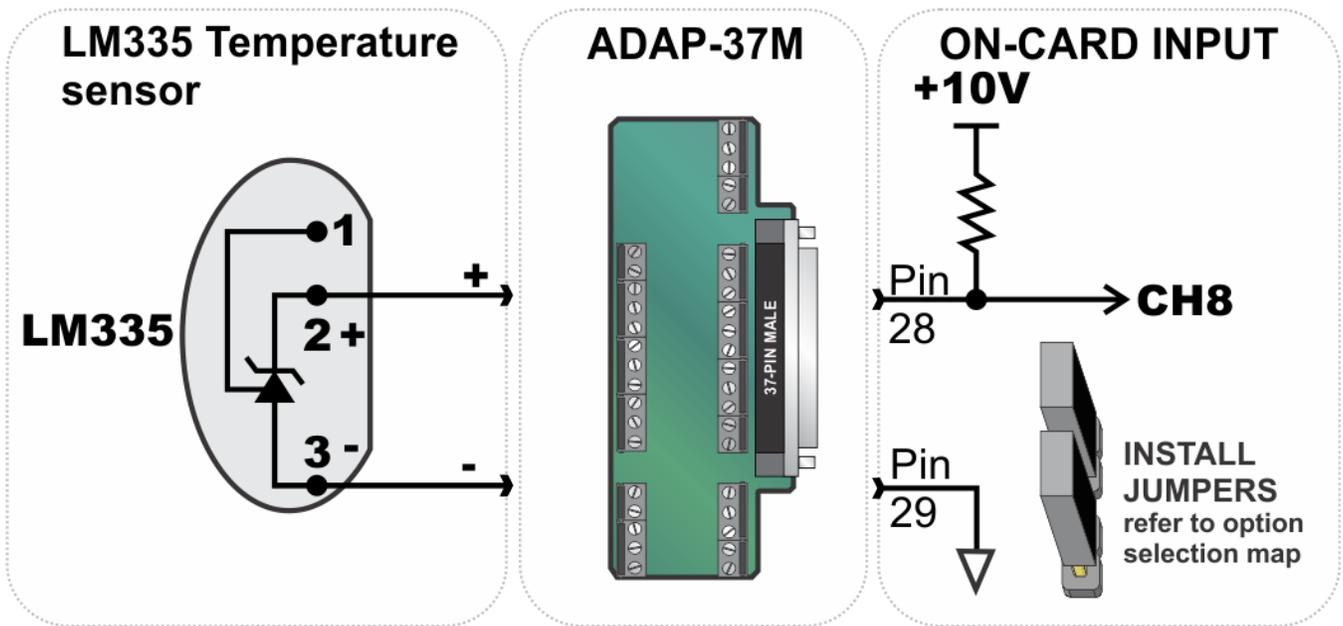
Figure 9-8: AIMUX-32 Reference Junction Temperature Sensor Diagram
